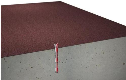
6. Using rotary hammer with SRA setting tool, install the AA402 eyebolt
