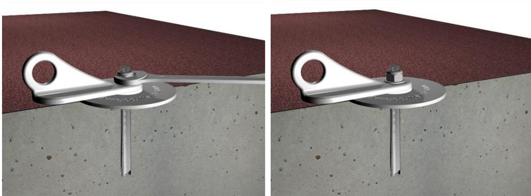
NOTE: When installing through water proofing membrane, a full gasket of quality polyurethane sealant is recommended between the base plate and the membrane.
