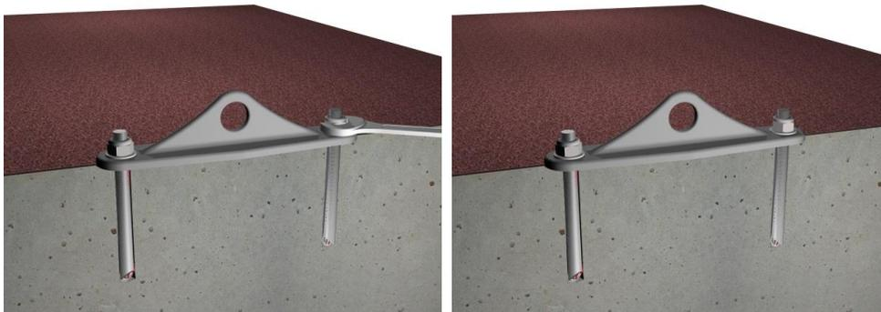
NOTE: When installing through water proofing membrane, a full gasket of quality polyurethane sealant is recommended between the anchor base plate and the membrane.
