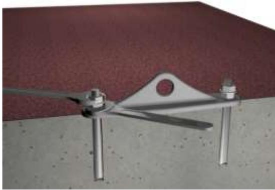
8. Install one M12 washers and one M12 nylock nut on each rod ensuring minimum of 3 threads are showing when nuts are fully tightened.
