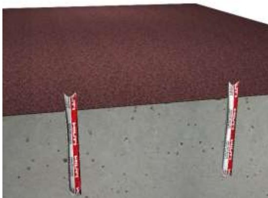
6. Using rotary hammer with appropriate setting tool, install 2 stainless steel M12 rods through the holes in the base of AA408 anchor. The rods must have their tips cut on 45° angle to allow for correct mixing of chemical.
