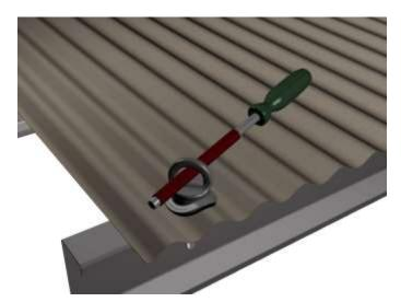
NOTE: The neoprene seal will work better on a clean roof. In case the roof is not in a clean condition, it may require some sealant under the neoprene seal. Clear sealant is required to be applied between the eye bolt and the base plate to ensure water proofing as well as prevention from seizing.
