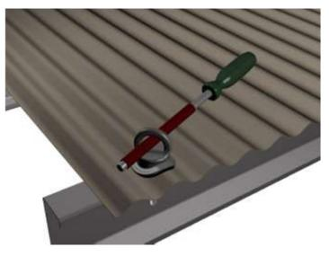
**Note:** The neoprene seal will work better on a clean roof. In case the roof is not in a clean condition, it may require some sealant under the neoprene seal. Clear sealant is required to be applied between the eye bolt and the base plate to ensure water proofing as well as prevention from seizing.
