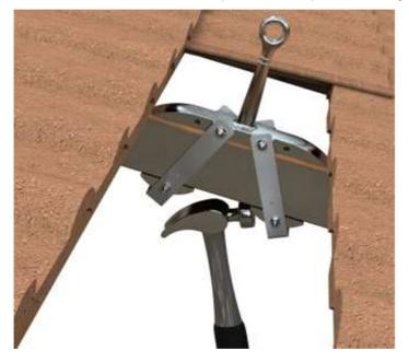
5. Install 2 small nails (provided) next to the friction plates to keep them engaged at all times.
