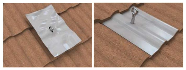
**9.** Apply polyurethane sealant under the Roof-tite flashing (provided) and shape the base of the flashing to adhere to the tile's shape perfectly.
