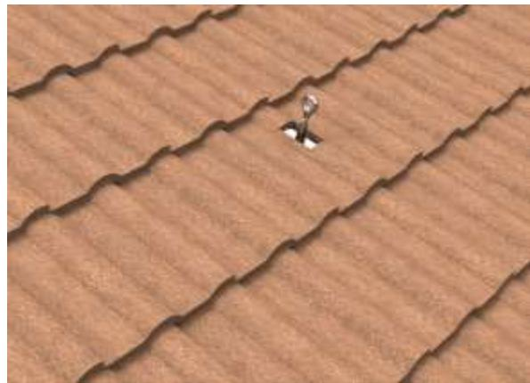
8) Apply Wakaflex or similar flashing over the tile and cut to size with Stanley knife.
