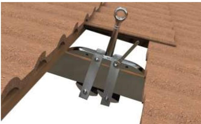
4. Use a hammer to knock the friction plates into compression and tighten the bolts.
