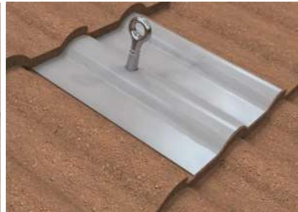
9) Apply polyurethane sealant under the Roof-tite flashing (provided) and shape the base of the flashing to adhere to the tile's shape perfectly.
